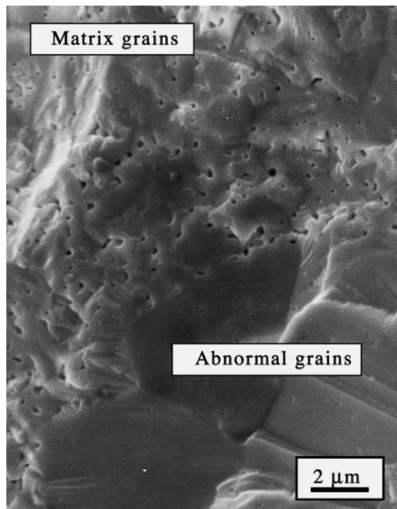
Fig. 12. SEM fracture surface of \text{UO}_2 doped with 0.25 wt% \text{Cr}_2\text{O}_3 , showing the development of dense abnormal grains inside a fine-grain matrix.
